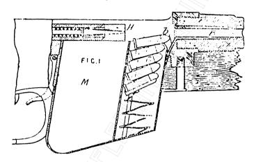
Adapting for miniature-ammunition practice; magazines.—A breech tube B fits the chamber of the gun and has a projecting tail b to keep it in position. The bolt head H carries a special extractor to suit the small cartridges. A special magazine C to contain the miniature cartridges is carried in the fore part of the magazine M.
